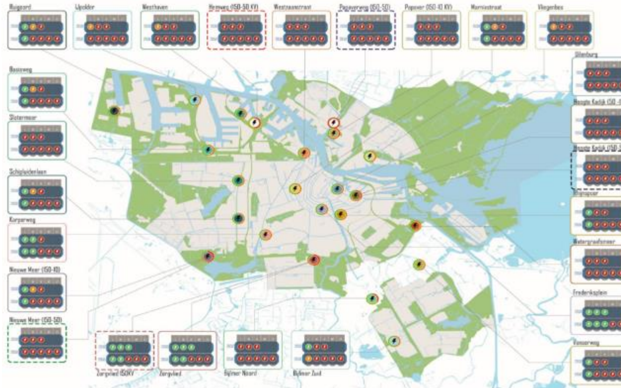
Substations in Amsterdam, red lights indicate capacity is insufficient (Liander, 2019)
